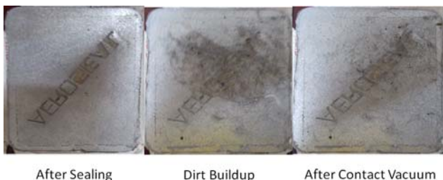
Figure 5: Source removal is impossible after sealing.
